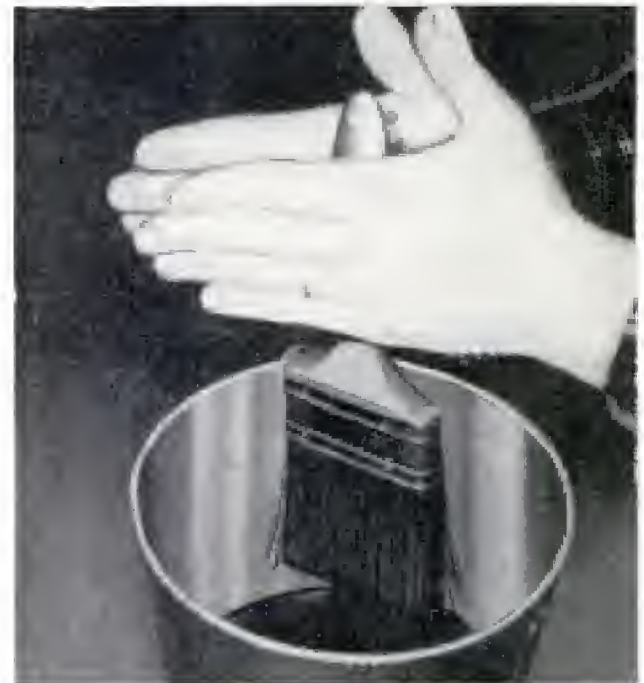
After soaking new brush in linseed oil for 24 hrs., it is spun dry by rolling rapidly between palms. Brush is held well down in empty pail for spinning
